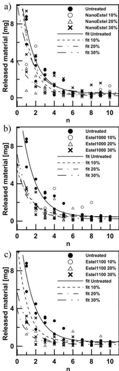
Figure 7. Results of peeling tests performed on a) NanoEstel-, b) Estel 1000-, and c) Estel 1100-treated samples. A set of three measurements had been carried out for each treatment; curve calculation had been performed by taking into account all data.
