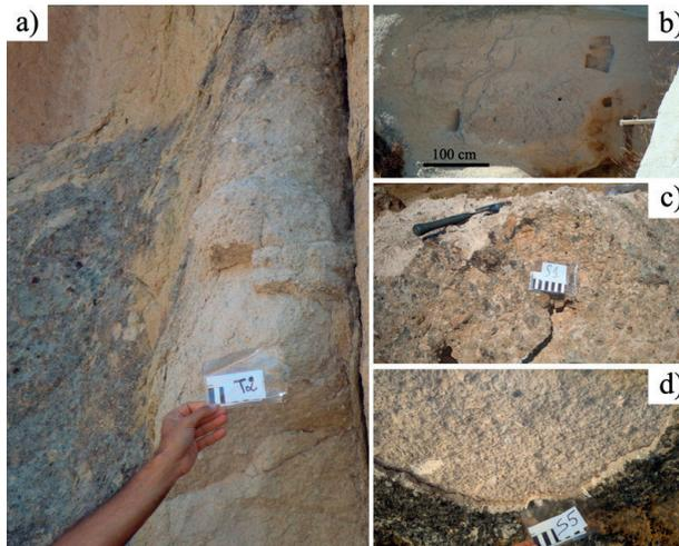
Figure 3. Sampling locations and related degradation forms for: a) sample T2 (lichen colonization and exfoliation); b) sample T1 (exfoliation and reddish colouring); c) sample S1 (detachment); d) sample S5 (scaling and soiling).
