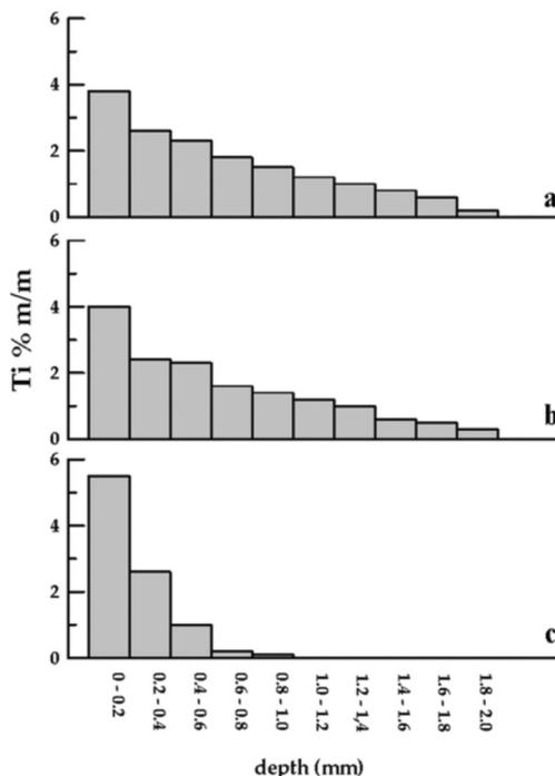
Figure 5. Ti distribution from the surface to the stone bulk for Estel 1000 (a), Estel 1100 (b), and NanoEstel (c). Ti content reflects the consolidant penetration depth.
