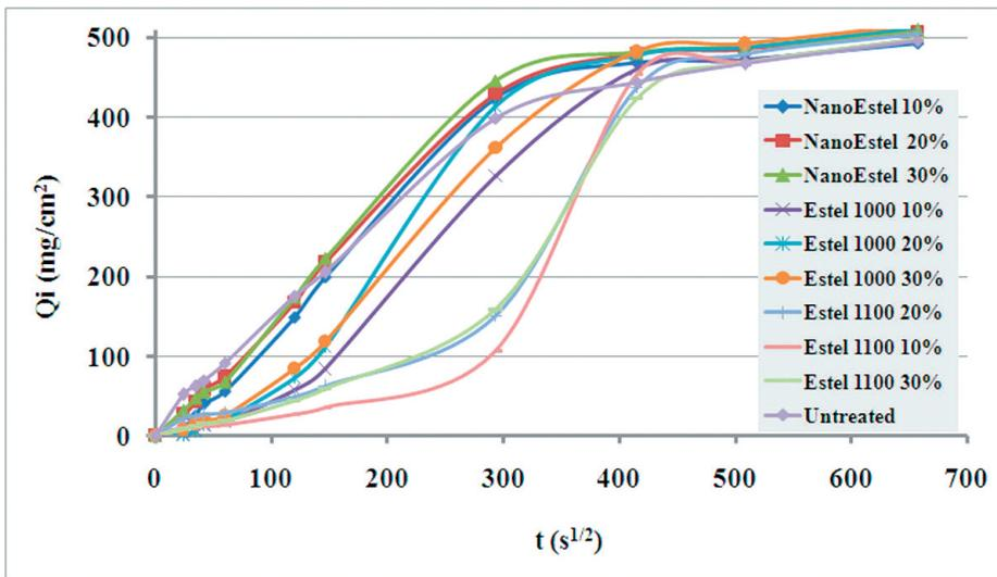
Figure 6. Capillary water absorption of treated and untreated specimens (x-values are expressed as the square root of seconds). Experiments had been carried out up to 5 days (~ 657 s<sup>0.5</sup>).
