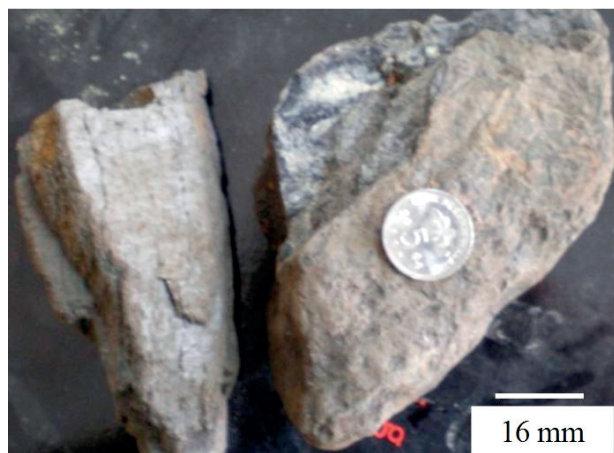
Figure 3. Visual assessment of Malaysian low-grade manganese ore (LGMO) samples obtained for this work.
