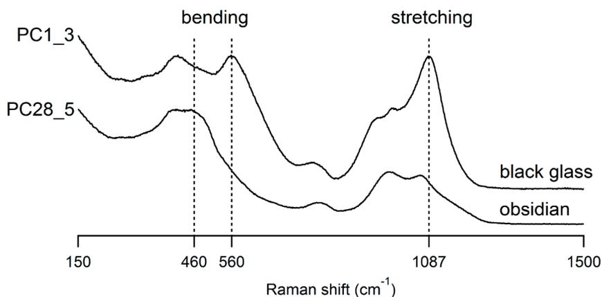
Figure 4. The Raman signal of a Roman black glass (Low magnesium glass, high iron) and a natural obsidian glass (Carthage). The bending modes are more relevant in obsidian than in man-made glass (peak at  $460 \text{ cm}^{-1}$ ). On the contrary, the stretching band at  $1087 \text{ cm}^{-1}$ , due to  $Q_3$  species is more prominent in Roman glass. The band at  $560 \text{ cm}^{-1}$  is due to bending motions of depolymerized network.
