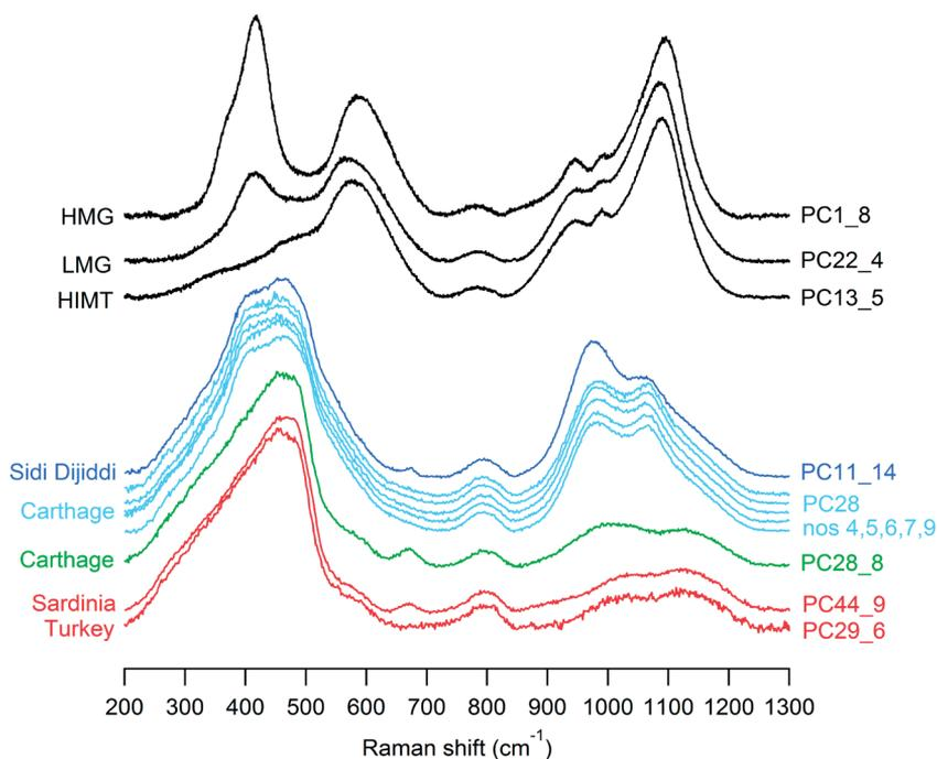
Figure 5. Raman spectra of Roman obsidian and man-made glass from different locations. When compared with Fig. 2 it is clear how the bending modes peak at  $460\text{ cm}^{-1}$  are evident and the stretching band at  $1087\text{ cm}^{-1}$  is lower than in man-made glass. Examples of Raman spectra of black Roman glass can be found in Baert et al. (2011).
