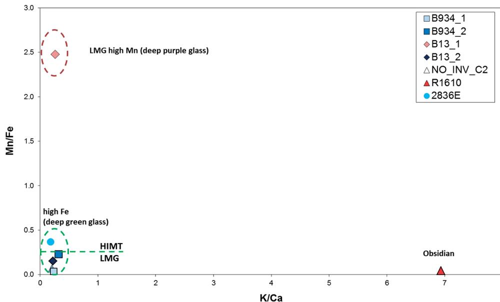
Figure 3. Plot of the Mn/Fe versus K/Ca ratios (results based on semi-quantitative micro-XRF) of R1610 and other Roman man-made glass. The Mn/Fe ratio identifies the Mn purple-coloured glasses from the Fe-green coloured. A K/Ca ratio lower than 0.3 is typical for Roman man-made glass, while a K/Ca ratio of 7 is characteristic to obsidian.
