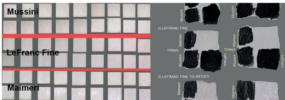
Figure 2. Specimens of white and application of black layer then 15 days (macro).
