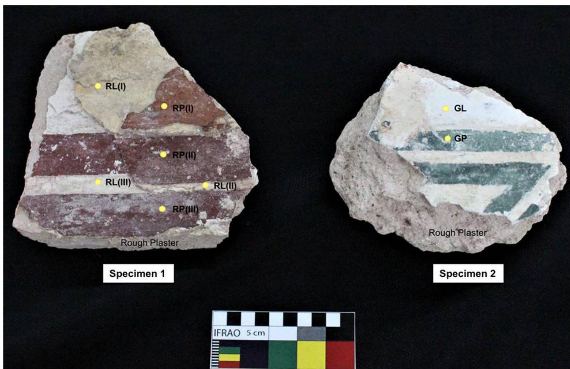
Figure 3. Fragments from the decorative wall of Chhatta Chowk, where RP(I) red first pigment layer, RP(II) red second pigment layer, RP(III) red third pigment layer, RL(I) first plaster layer of RP(I), RL(II) secon.
