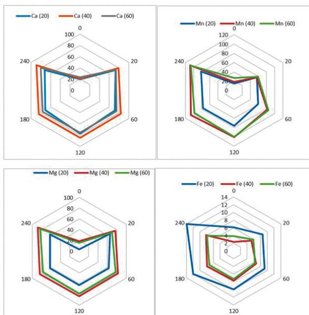
Figure 3. Leaching results of the Ca, Fe, Mg and Mn elements with 2 M HCl.
