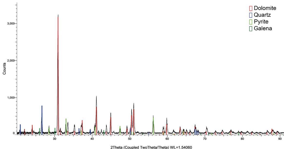
Figure 1. XRD pattern of mining flotation tails.
