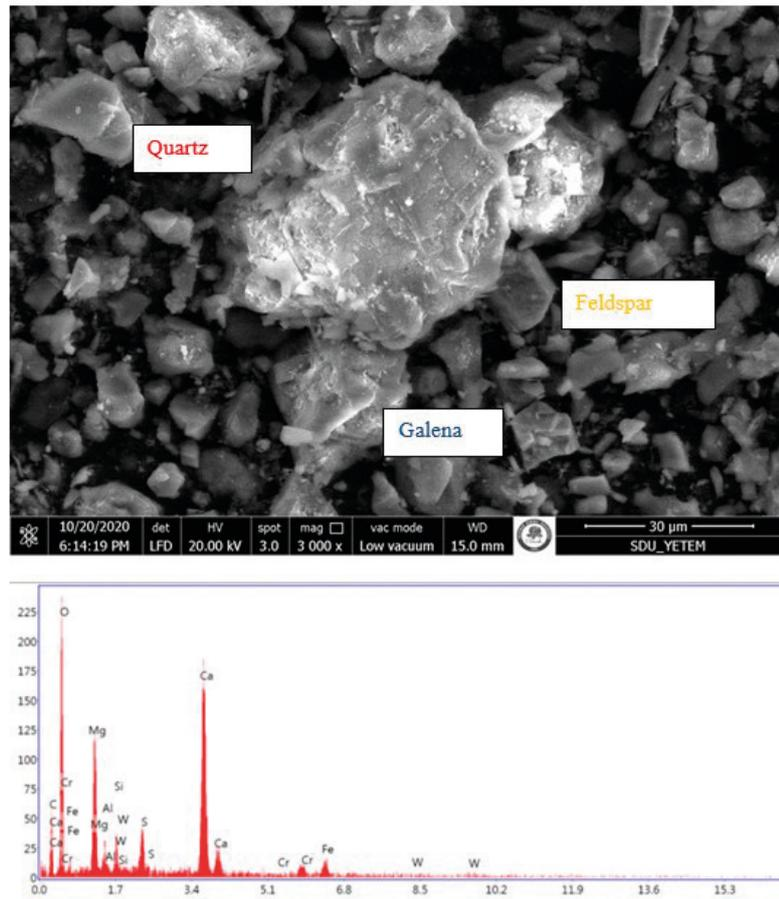
Figure 2. SEM-EDX image of mining flotation tails.
