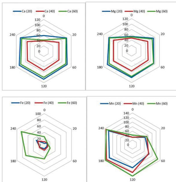
Figure 6. Leaching results of the Ca, Fe, Mg and Mn elements with 2 M  $\text{HNO}_3$  and 2 g/L citric acid.
