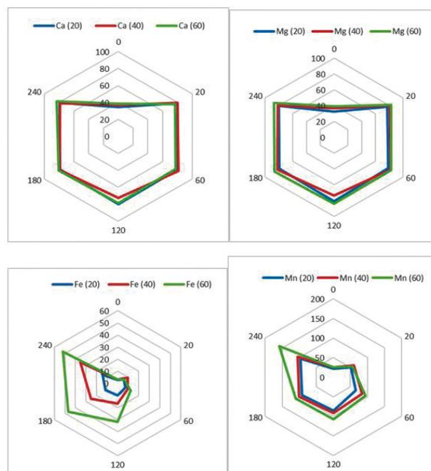
Figure 5. Leaching results of the Ca, Fe, Mg and Mn elements with 2 M  $HNO_3$ .
