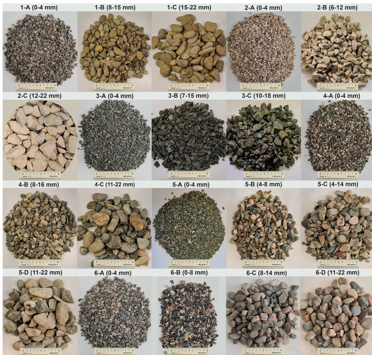
Figure 1. Macroscopical picture of various grain-size fractions of aggregates investigated.
