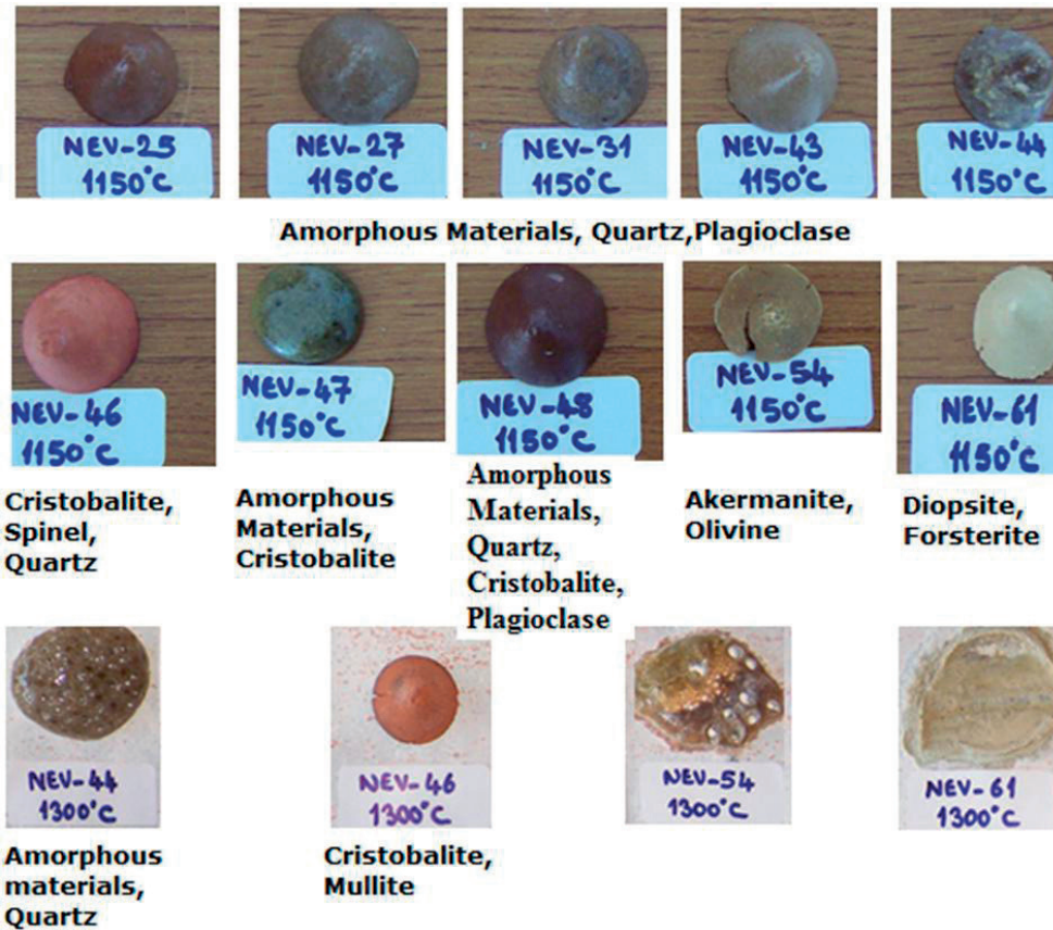
Figure 14. Firing conditions, colors and mineral developments of samples fired at 1150 °C and 1300 °C.
