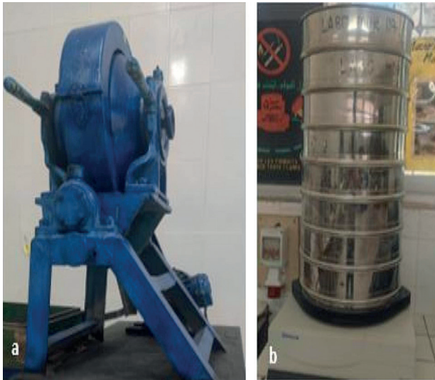
Figure 2. Laboratory equipment used in the grinding experiments. a) laboratory-scale ball mill used for grinding tests; b) RETSCH vibratory sieve shaker used for particle size analysis.
